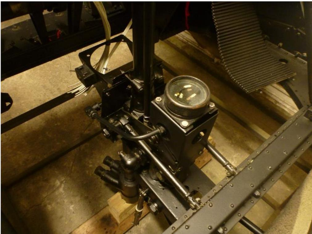
The plan for April is to get working on the plethora of hydraulic components and small detail items that connect the turret control unit to the servo feed unit, hydraulic motors and elevation ram. This is going to be a fiddly process but at least the weather is now getting warmer and the workshop is more comfortable.
