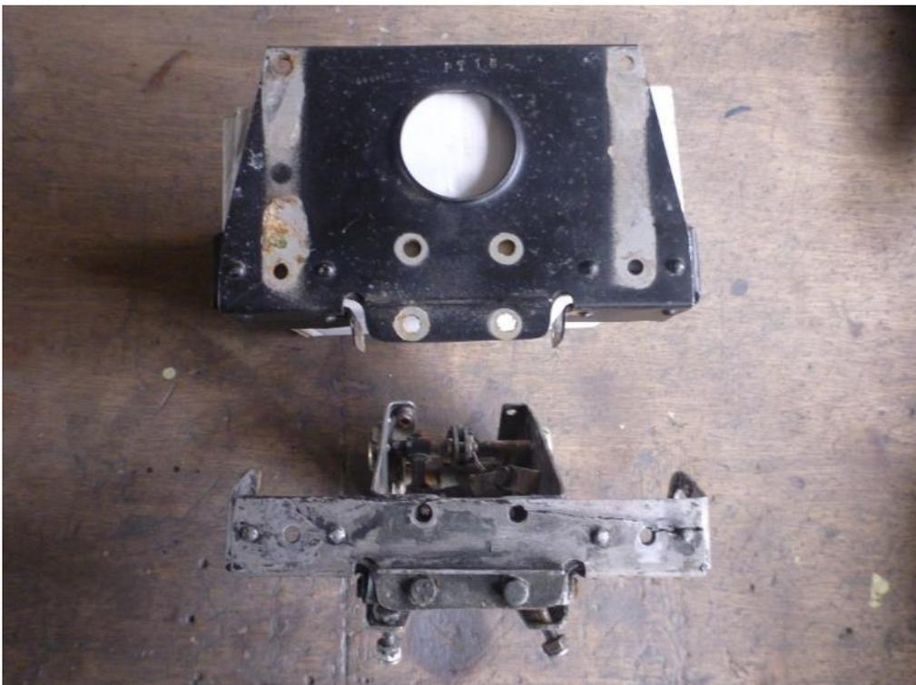
With the turret control units completed as far as possible, there was still time in March to launch into the control panel. Although in not too bad condition, the panel had been modified over the in-service years. With the panel stripped back it was possible to clean up and re-spray it and then identify the components that were fitted in accordance with the original Air Publications.
